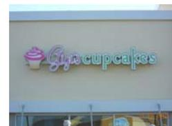
2. Back Lit. The idea with back lit signs is to create negative space for the lettering. If the face is not translucent, but opaque, and the neon in the can is designed to illuminate the wall behind the sign instead of the letters themselves, the letters appear as darker shapes against a field of light, a very interesting look.
